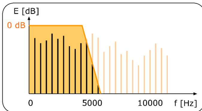
example of band-limiting of a typical signal
